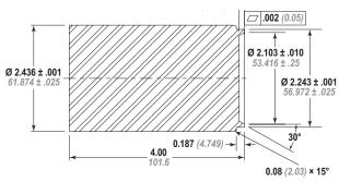
MATL P/N: CR1215RO-0250 × 4.25 (88.9) LG COLD ROLLED STEEL BAR Ø 2.50 (63.5) OD × 4.25 (107.95) LG
