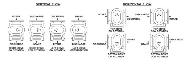
Figure 4-2 – Flow Direction by Rotation
