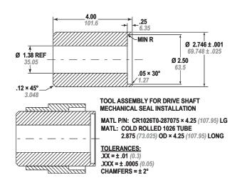
Figure 13-3 – 4000/5500 Seal Pressing Tool (T11449-1)
