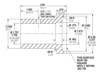
Figure 13-4 – 4000/5500 Pressing Tool for Mechanical Seals
