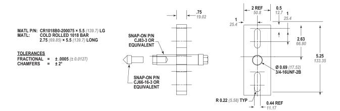
Figure 13-5 – 4000/5500 Gear and EP Tool (T29603)
