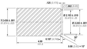
MATL P/N: CR1215RO-0250 × 4.25 (88.9) LG COLD ROLLED STEEL BAR Ø 2.50 (63.5) OD × 4.25 (107.95) LG
