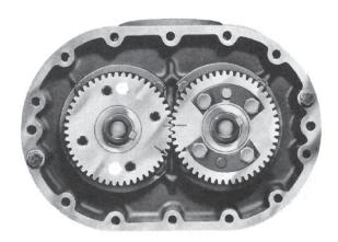
Figure 8-3 – Timing marks advanced 3 teeth (reference marks aligned)
