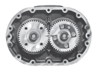
Figure 8-2 – Keyways in line and timing marks matched
