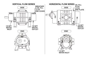
Figure 5-4 – Water Cooling Connections
