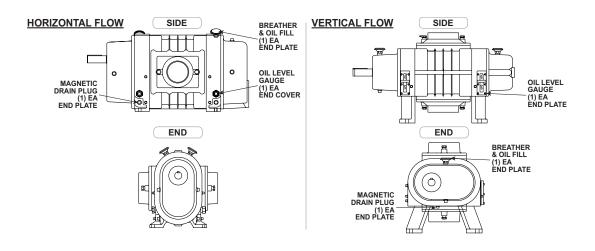
Figure 5-3 – Oil Fill, Drain Connections, and Oil Level Gauges
