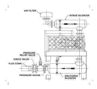
Figure 5-1 – Typical Blower Installation
