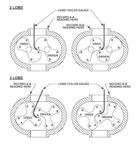
Figure 8-4 - Checking Rotor Interlobe Clearance
