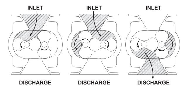
Figure 4-1 – General Operation Principle
